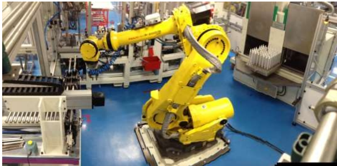
Rack Protector Robotized Washing Cell
