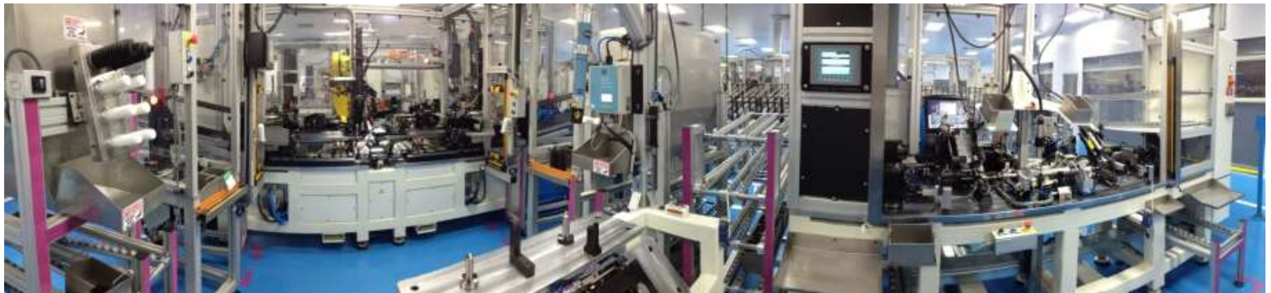
Outer , Inner Balls and Bellows Assembly Process
