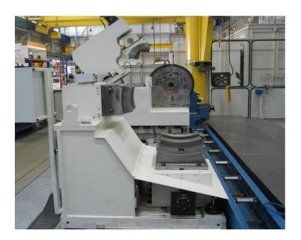
**Development of new study rests for** generator shaft slot milling machine, including upgrading of the machine to **CNC** technics.
