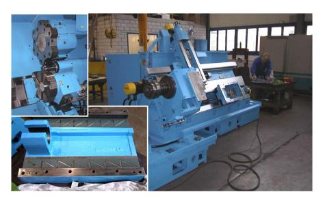
The Nakamura CNC – controlled turning machine was mechanically and electrically completely overhauled, including grinding of the guide ways and remade of the geometry. After the retrofit the machines was delivered to the customer with new machine warranty.
