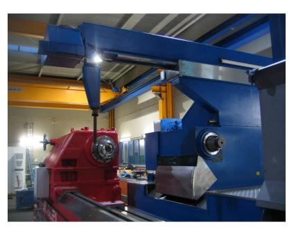
New roll measuring system, conversion to CNC – technics, upgrading grinding spindle power up to 260 Kw
