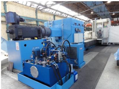
Complete mechanical and electrical overhauling of the Herkules roll lathe including upgrading to CNC - technics
