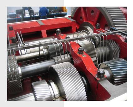
Retrofitting of gear box of roll turning machine including approx. 50% new gears.
